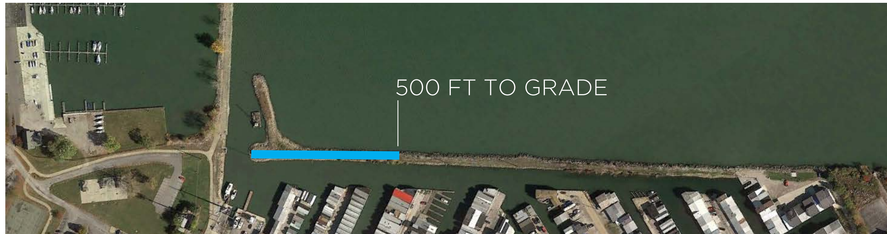
PIER TRACK BRIDGE: Several bridge designs and heights were considered during the development of the Pathway Update. After determining that a movable bridge would potentially be a long term maintenance concern, consensus was reached that a fixed bridge with a 25-foot vertical clearance balanced the needs of the marine community, typical vessel heights for Lake Erie, and the desire to bring the Pathway along the waterfront.
